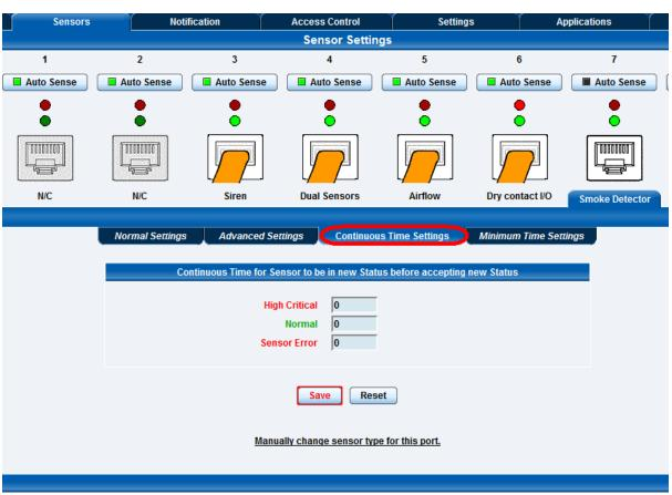
Again, as we mentioned before at the end of the sensorProbe configuration, when we tested the smoke sensors, we found that if these are positioned too close to the florescent lighting, these lights can cause false alerts. You can add time to the "Continuous Time Settings" as shown in the screen shot above to eliminate these false alerts.
