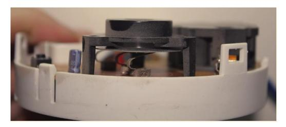
The picture above clearly shows the dust build up inside the detectors optical chamber. You can see the clear black plastic where we have wiped the dust off compared to the dusty surface.
