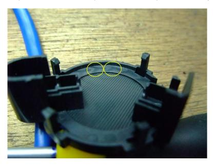
This picture above also shows the dust inside the cover of the Smoke Detector.
