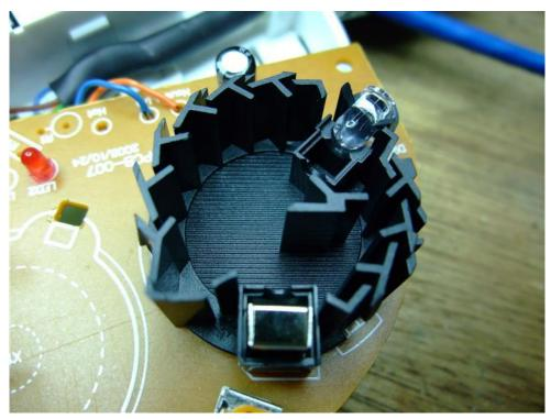
This picture above shows the optical chamber of the Smoke Detector after cleaning
