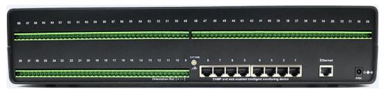
The rear view of the sensorProbe8-X60 shows the 60 dry contact inputs, the 8 intelligent sensor ports, the 10/100 Ethernet port, the 5VDC AC power input jack and the GND ground stud.
