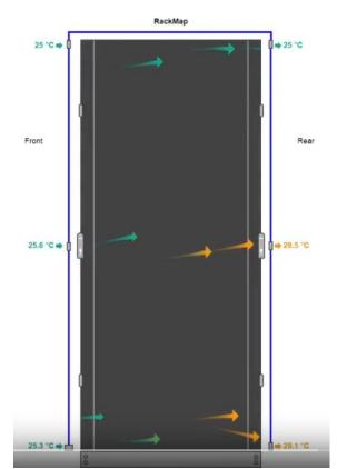
The Rack Map feature was originally (and still is) included in the AKCess Pro Server / AKCPro Server (HTML5) and has also been added to the SP+ units. You can add a Rack Map as a graphical representation of your server rack, and to display and record the temperature of the airflow within your server cabinets.
