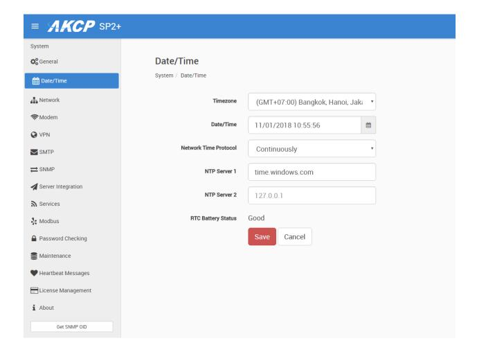
The system date and time with time zone is user configurable, with NTP server synchronization. If the unit is connected to APS (AKCPro Server), then it will sync with the APS NTP service. Also displayed is the status of the RTC battery (good/bad).
