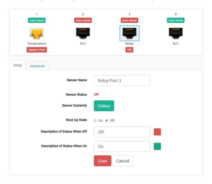
Boot Up State: You can change the state of the relay when the unit starts. The default is Off.
