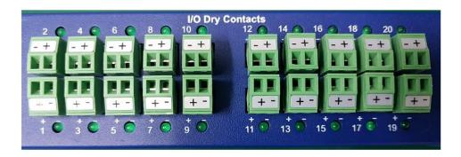
It is very important to take note and correctly connect the polarity of the connections as you can see in the image above as the two rows have a different orientation.
