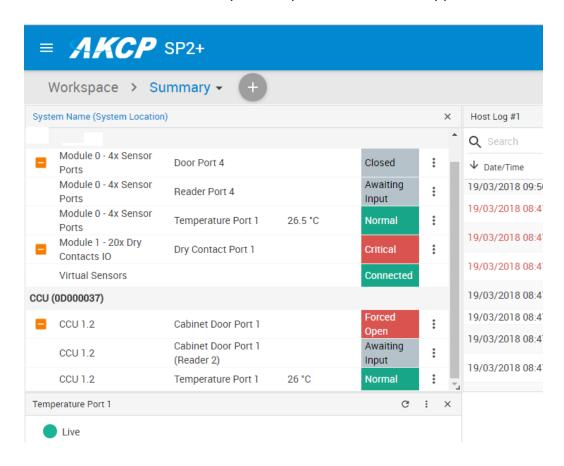
In the picture above we have a CCU (Cabinet Control Unit) connected as an expansion board, with an additional Temperature Sensor connected to one of its ports.
