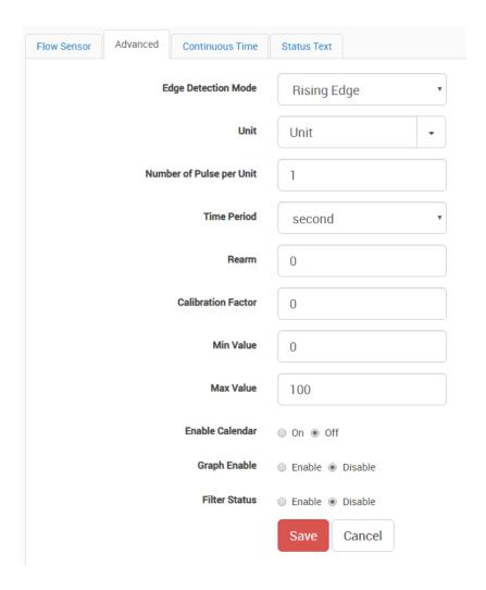
In the Flow Sensor there is "Number of Pulse per Unit" in the config. You can use this value to adjust the sensor reading to match the real-world value.
