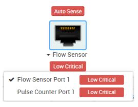
To set it up, disable Auto Sense on a sensor port and select the Pulse Counter sensor type from the list. This will give a dual sensor with Flow Sensor and Pulse Counter.
