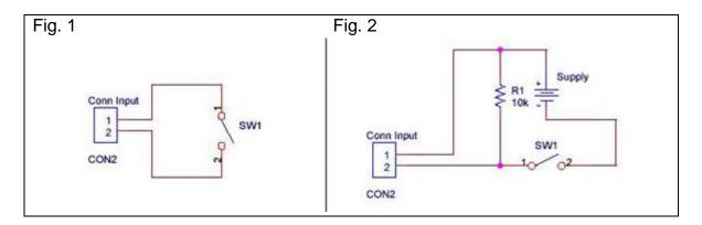
The standard Dry Contacts are as in Fig. 1: directly connected to the unit's controller board. In this setup, power is provided by the sensorProbe+ to the switches. With the sensorProbe+ providing the power, the switch has +5 Volts applied to pin 1 and GND applied to pin 2. When the switch is open, the input senses +5. When the switch closes, the input senses GND. No additional external power is needed.
