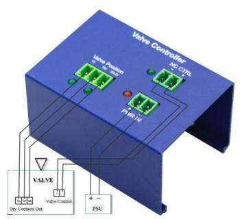
If you have DC motors or electronically controlled ball valves which require polarity reversal to turn in the opposite direction, this module is applicable. Ideal for water irrigation or industrial applications which require valve and motor controls.
