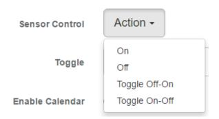
This button allows you to manually control the relay by controlling the cycle of the relay in an on-offon or an off-on-off cycle. You can also set the "Toggle" (Cycle Time) here in seconds.
