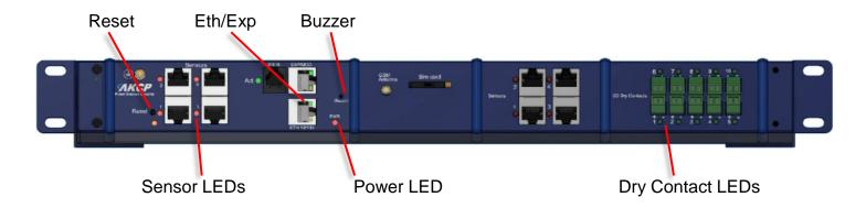
The **Ethernet/Expansion LEDs** have standard indication LEDs for network activity and connection state (green and orange).
