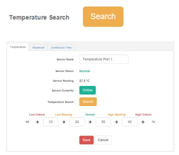
What this button does is to search for new temperature sensors in a chain, if you've connected more than 1 sensor in a Daisy-Chain Temperature (DCT) sensor chain.
