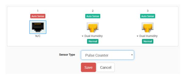
The sensor is designed to be used by disabling the Autosense and connecting an external sensor to the sensor port. This sensor will detect changes on the Data pin (Pin 1 of Sensor Port).
